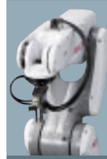
Conventional wrist overhanging cables
